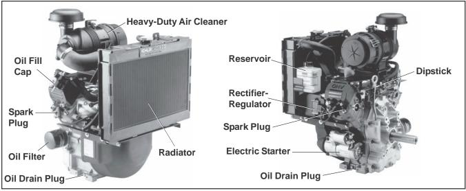
Figure 1. Typical Kohler Aegis Carbureted Engine.
